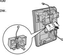
Install screws using the wall template below. Connect the telephone line cord. Mount the unit, and slide down.
