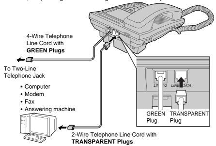
If the LINE2/DATA indicator lights red, the communication device is in use. Use LINE1 to make or answer other calls. Otherwise the communication device may not operate properly.
