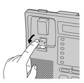
Tuck the telephone line cord inside the wall mounting adaptor, and push it in the direction of the arrow.
